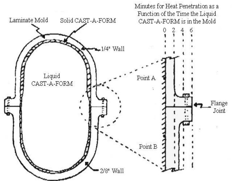
If the flange type joint should create a problem, one solution is to build the mold with lap joints fastened by quick closing clamps as indicated here. In places where the mold cannot be uniform in wall thickness, such as in throat areas, metal inserts can be used to bleed off the heat and enable **CAST-A-FORM** to build up in thickness uniformly with the rest of the mandrel.
